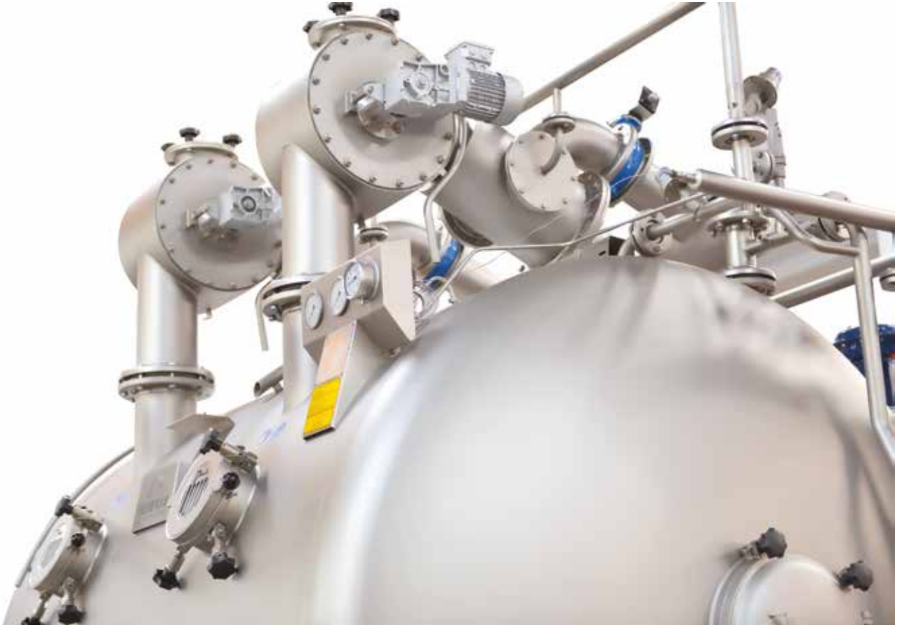
Motorlu Redüktör tahrikli kule sistemi (gear box) Gearbox driven main winch system
